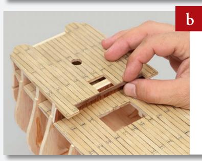
Cut a length of the wooden strip to fit the position shown in the photo. Glue it into place.
