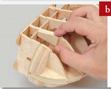
Glue the two bow frame reinforcements in place on Frame 2, under the main deck, one on each side.
