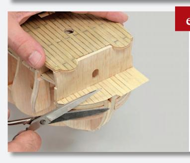
Once the planks are dry, cut off the parts that extend past the edge of the bowsprit deck.
