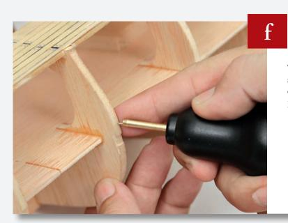
To test the pin pusher, load it with a nail, place the point against the centre of one of the frames and push forward.
