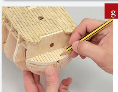
Mark the edges of the planks, as shown. There is no need to simulate the nails.
