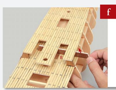
Glue bulkhead B into place under the stern deck, resting up against the bow side of Frame 9.
