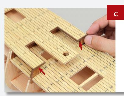
File the edges highlighted in the photograph, then cut another two lengths of the wooden strip and glue into place, as shown.
