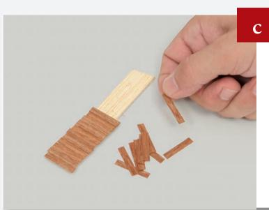
Cut the planks into short lengths and glue them onto the bulkheads.
