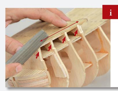
Begin shaping the hull frames, above the ledges on Frames 1-4, so that they are in line with the forecastle.
