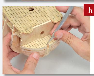
Using a knife, remove the strip of plank that covers the notch in the bowsprit deck, as shown in the photo.
