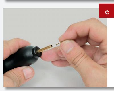
When using the pin pusher, always make sure that you insert the nail head first.
