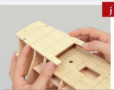
Once complete, glue the poop deck in place, resting on top of Frames 12-14.
