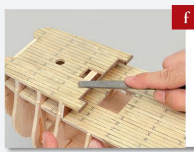
Check that the strips are flush with the planks of the forecastle deck, and file if necessary.
