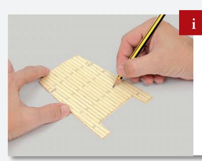
Prepare the planks as before and glue them onto the poop deck. When dry, cut off any planking that extends past the edge of the deck. Then mark points to imitate the nails.
