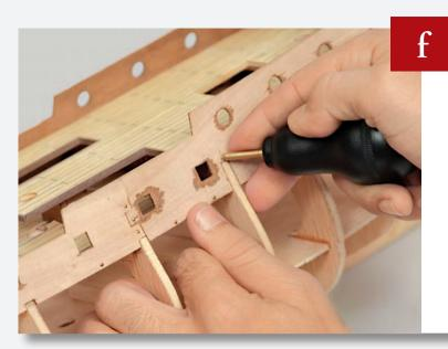
Apply glue to all contact areas, and while it's drying, nail the wall into place.
