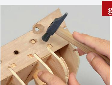
Once you have all the nails in place, gently tap them down with a hammer so their heads sink into the wood, making the outer surface level.
