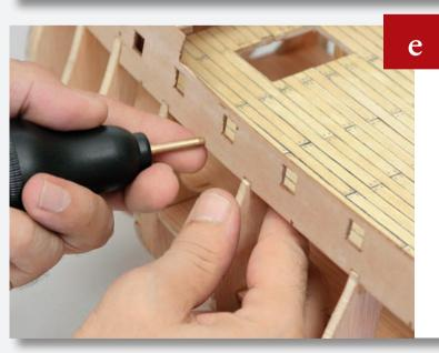
At the narrowest point of the side wall, nail along the bottom edge to join it with the main deck.
