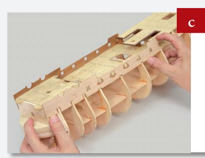
Test-fit the side wall up against the hull. If you have trouble fitting it up against these frames, sand or file the slots slightly until it fits.
