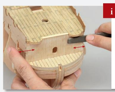
Smooth the edges of the side walls until they are flush with Frame 1.
