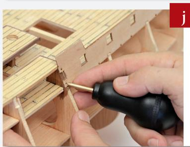
At the end of the side, where it doesn't cover the deck, nail it only to the frame.
