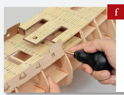
The aft end of the port side wall should finish at the same height as the starboard wall.
