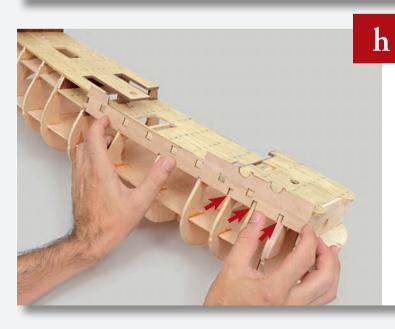
Test-fit the side wall up against the hull. If you have trouble fitting it up against these frames, sand or file the slots slightly until it fits.
