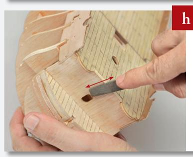
Once the glue is dry, file or sand off the overhanging plank until it is flush with the bow bulkhead, Frame 1.
