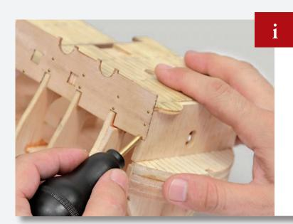
Apply glue to the areas of contact and start nailing the ship's side to the hull. Begin at the bow and continue towards the stern.
