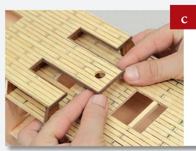
Cut another piece of the strip to cover the front edge of the deck. Glue into place.
