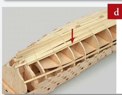
Glue and nail a plank into place from Frame 8 to Frame 13.
