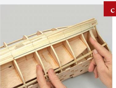
Once the last plank has dried in place, glue and nail another from Frame 8 to past Frame 13. Repeat Steps a-c for the other side of the hull.
