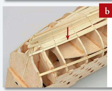
Glue and nail another plank to fit from Frame 11 to Frame 14.
