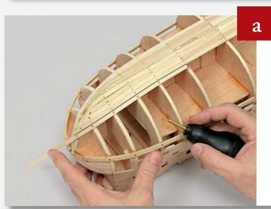
Take a plank and place it halfway across Frame 5. Glue and nail it into place up against the next plank. Once the glue has dried, cut away the area of the plank that overlaps the false keel.
