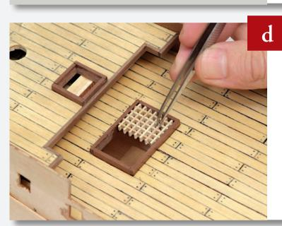
Glue the 18 x 23mm grating into the larger hatch on the main deck at the bow.
