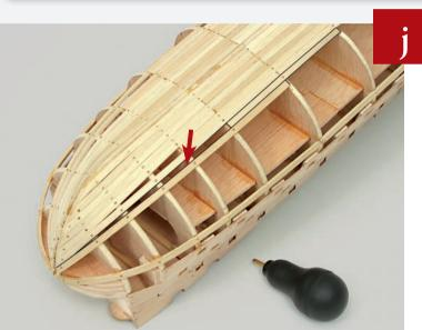
Now glue and nail another plank to the hull, this time to fit from Frame 6 to the bow.
