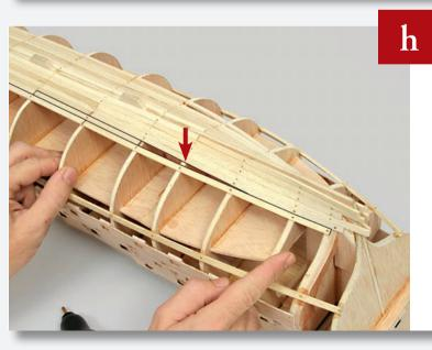
Glue and nail another plank from Frame 8 to Frame 13. As with Step f, this will create a wedge-shaped gap.
