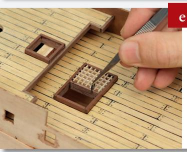
Cut a length of 2 x 7mm wooden strip to fit in the centre of the hatch, next to the grating you fitted in the last step.
