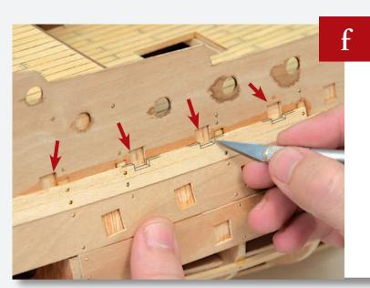
Use a knife to remove any parts of the planks that block the gun port openings.
