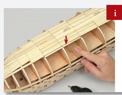
Shape a plank to fit from Frame 5 to Frame 7, then glue and nail it into place.
