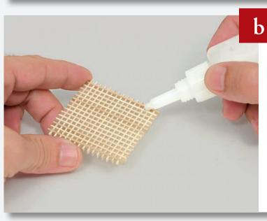
Apply adhesive to all the joints so that the grating becomes one single piece.
