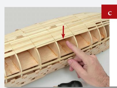
Glue and nail a plank to fit next to the plank fitted in Step j, Page 116, to run from Frame 6 to Frame 8.
