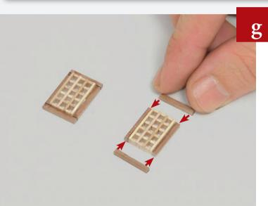
Using the photograph as reference, cut and glue lengths of the  $2\ x$  2mm wooden strips to fit around the sides of the  $11\ x\ 18$ mm gratings.
