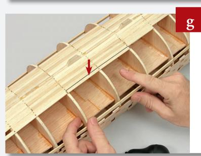
Continuing aft of the plank fitted in the last step, glue and nail another into place, from Frame 6 to Frame 8.
