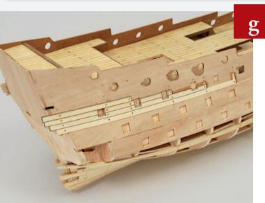
Continue to fix planks to the bulwark at the stern. One should run from Frame 11 aft, another from Frame 12 aft. Remember to remove any part of the planking that covers the gun port holes.
