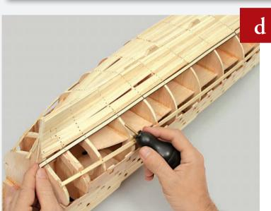
Glue and nail into place a further two planks, one running from Frame 6 to Frame 10, and another from Frame 10 aft.
