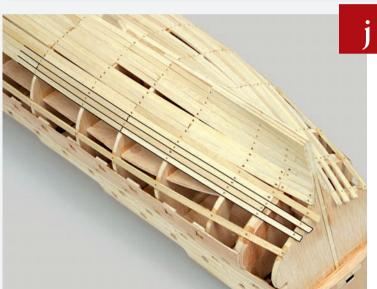
Note how the planks are arranged at the stern of the hull.
