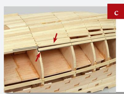
Continue to nail the plank to the frames, with it finishing at Frame 6 next to the plank on its side from Step a.
