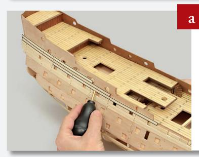
Add more planks to the bulwarks, continuing up from Page 123, as shown. Add nails where you can, and where you cannot, use a quick-setting glue such as superglue.
