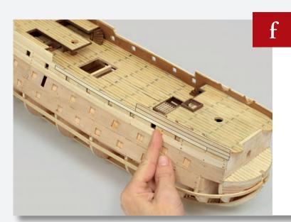
Continue forward, adding planks to cover the bow bulwark. Repeat for the other side of the hull.
