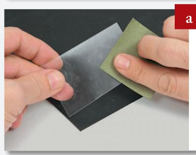
Lightly roughen the surface of the acetate sheet with sandpaper on both sides.
