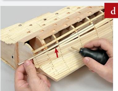
Glue and nail another plank into place, from Frame 10 to Frame 14, creating another wedge-shaped gap.
