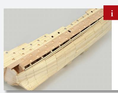
Fit two planks running from Frame 5 to Frame 8 and then from Frame 8 to Frame 13.
