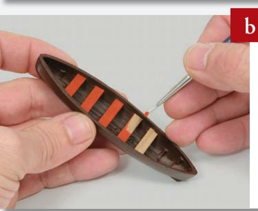
Cut the wooden strip into five lengths and glue them into place inside the boat. Paint the lengths of wooden strip red.
