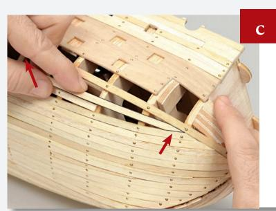
Shape a plank to fit in the gap at the bow, as shown, ending at Frame 5.
