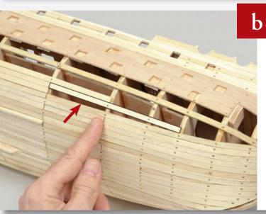
Place another plank below the last one, from Frame 6 to Frame 3, creating a wedge-shaped gap.
