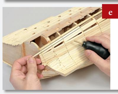
Glue and nail a plank above the one from the last step, from Frame 11 to Frame 14.
