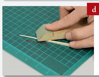
If necessary, use sandpaper to reduce the wedge to the size of the gap.
