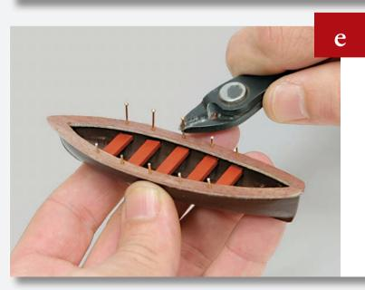
Glue nails into the holes, keeping them vertical while drying. Cut the tops of the nails off approximately 4mm from the base.
