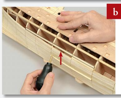
Cut and glue another plank to fit from Frame 6 to Frame 10, creating a wedge-shaped gap.
