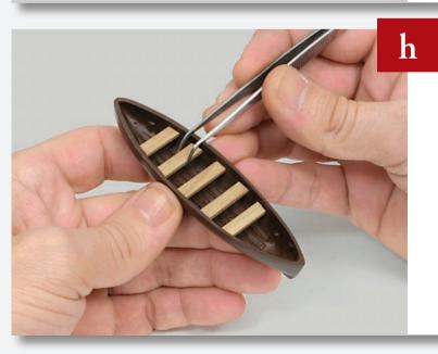
Cut the wooden strip into five lengths to fit the hull and glue into place inside the boat, as shown.
