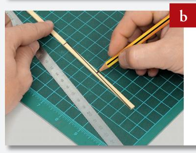
Draw a diagonal line from one corner of the marked area to the opposite corner, as shown.
