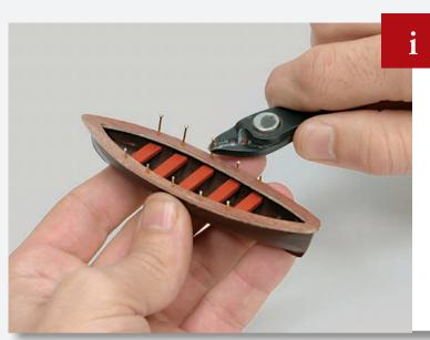
Cut the tops off the nails, approximately 4mm from the base to leave the shanks projecting as rowlocks.
