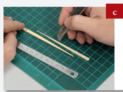
Carefully cut along the line to create a wedge-shaped piece. Test-fit it in the gap.
