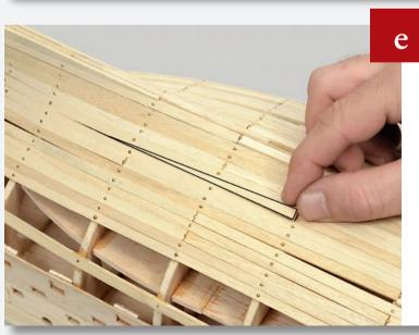
Keep testing the wedge until it fits exactly, then glue it into place.
