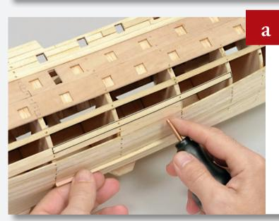
Continue to plank the hull. Glue and nail a plank to fit from Frame 5 to Frame 8.
