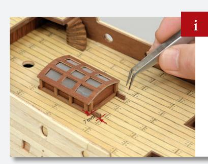
Cut two 7mm lengths of 2 x 4mm wooden strip and glue them in front of the skylight, standing on edge. Position them in line with the centres of the upright frames of the skylight.
