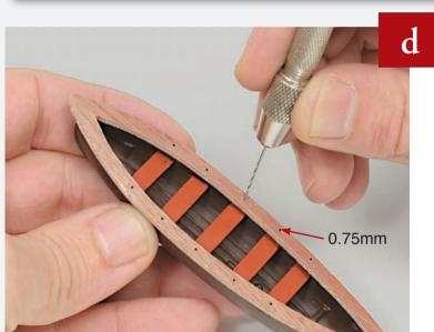
When the glue has set, drill holes in the centre of the bulwark, in line with the middle of each wooden strip, using a 0.75mm drill bit.
