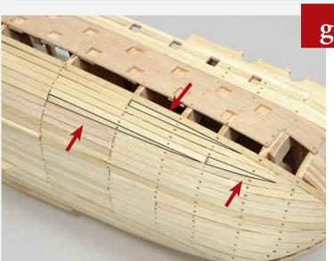
Use the technique from pages 145 and 146 to fill the gaps in the planking at the bow.
