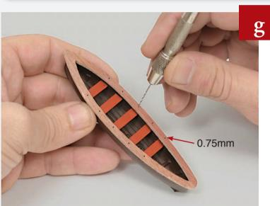
Take the boat assembly and drill holes through the centre of the bulwark, in line with the middle of each wooden strip. Use a 0.75mm drill bit.
