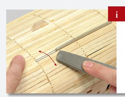
Once the glue has dried, file the surface flush with the rest of the planks, moving around the curve of the hull.
