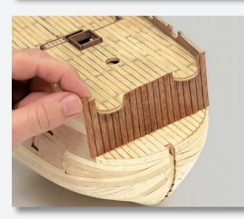
Glue planks to the bulkhead area of the bow, as shown in the photo.
