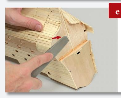
File the planks aft, so they are flush with Frame 14.
