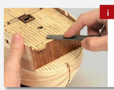
Cut away the excess plank ends at the top of the bulkhead and then smooth the edge.
