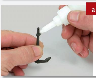
Apply a drop of superglue to the top end of one anchor shank.
