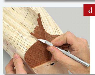
Continue to fill in the remaining space on the frame. When all the planks have dried, cut away the excess.
