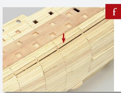
Locate any small gaps in the central section of the hull.
