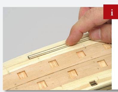
Take a plank long enough to cover the shallow area and glue it in place on top of the other plank.
