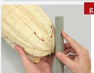
Smooth the hull at the bow, moving with the shape of the hull.
