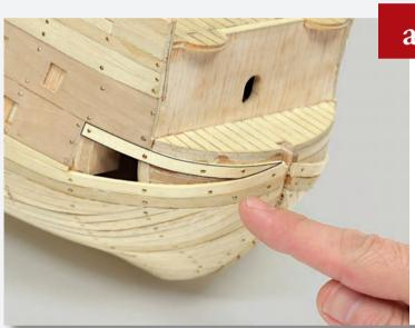
Shape a plank to fit from below the second row of bulwarks to the bow, as shown. Glue and nail it into place.
