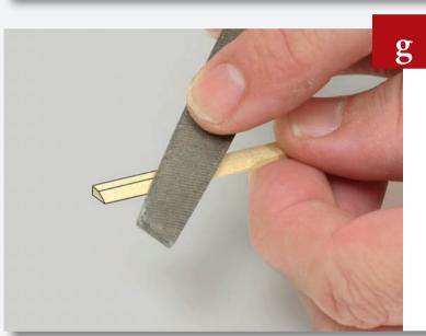
Take a plank the length of the gap you are trying to fill and file one edge into a wedge shape.
