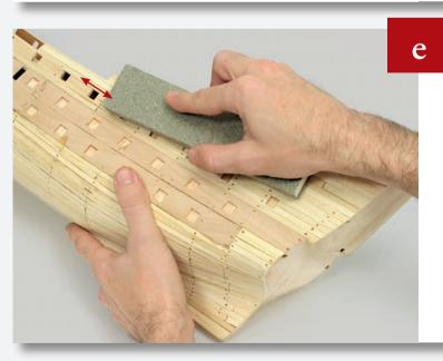
Smooth along the entire length of both sides of the hull.
