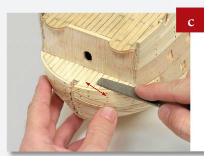
File the planks so they are aligned with the deck.
