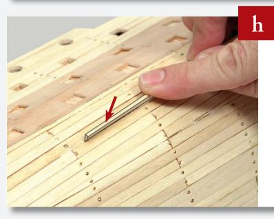
Now insert the plank into the gap and glue into place.
