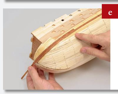
Place another plank above the one you fitted in Step b, running from the bow to Frame 4, and trim off the excess at the bow.
