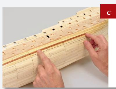
Continue from the last plank, gluing another plank in line with it and the upper planks.
