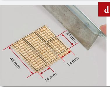
Position the grating as shown. Using the measurements in the photo, cut it into four pieces.
