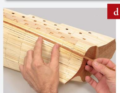
Glue a final plank into place, in line with the previous plank and running past the stern. Carefully trim the end flush with the stern.
