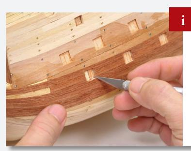
Continue to plank upwards, covering the port sides of the lower two gun decks. As you place the planks over the sides of the gun decks, remember to cut out the gun port openings.
