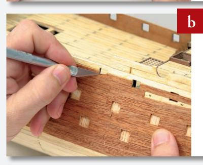
Remember to cut away any planks covering the gun port openings.
