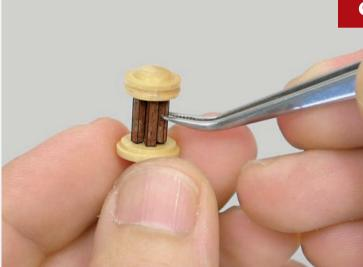
Cut the wooden strip into six lengths to fit in the gap between the two ends of the capstan and glue into place.
