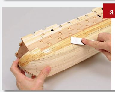
Apply glue to the surface of the upper planks on the port side of the hull, as shown in the photo, from bow to stern.
