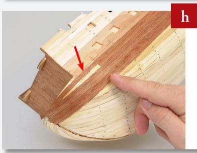
You will notice that it isn't always possible to keep the brown planks in line with the previous ones. It is better to try and match the shape of the hull rather than that of the previous planks, even if in doing so it creates gaps or overlap.
