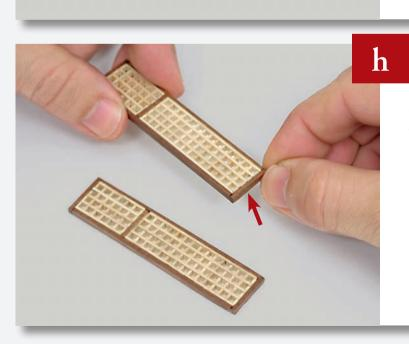
Then cut two 14mm lengths of the wood and glue to each end of the assembly. Repeat for the remaining grating pieces.
