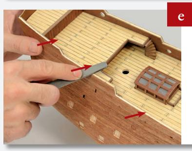
Gently sand or file the tops of the side walls on each side of the ship.
