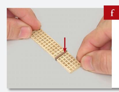
Take the 2 x 4mm strip of wood and cut a 14mm length from it. Glue this strip between a long and a short piece of the grating.
