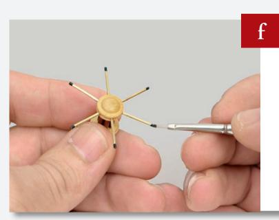
Cut the brass wire into six 2cm lengths. Glue them into the holes in the top of the capstan and then paint the ends black.
