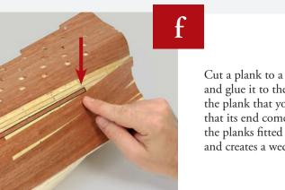
Cut a plank to a length of 210mm and glue it to the hull aft and above the plank that you fitted in Step e, so that its end comes into contact with the planks fitted earlier, as shown, and creates a wedge-shaped gap.
