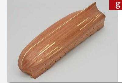
Continue to plank up to the horizontal planks at the sides, so that there are only the wedgeshaped gaps left.
