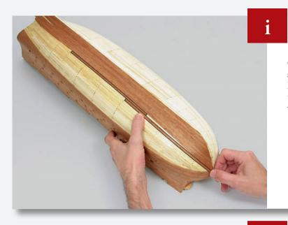
Glue a plank in place at approximately the centre of the hull's length, then glue one from the bow, as shown, creating a wedge-shaped gap.
