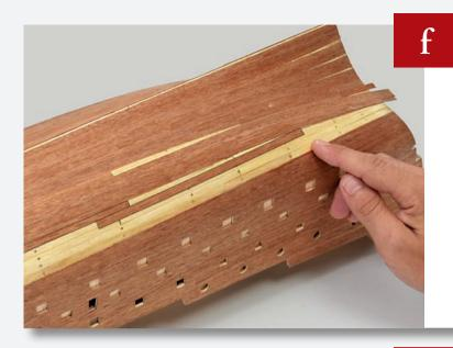
Cut a plank to a length of 210mm and place it aft and above the plank fitted in Step d, so that its end comes into contact with the previous rows and creates a wedgeshaped gap, as shown.
