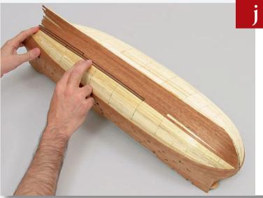
Next, glue a plank aft of the one at the centre of the hull, and then complete the row that you started with the plank fitted from the bow in the previous step.
