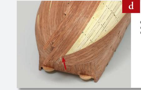
Continue to fit planks to the hull until they come into contact with those fitted earlier, as shown.
