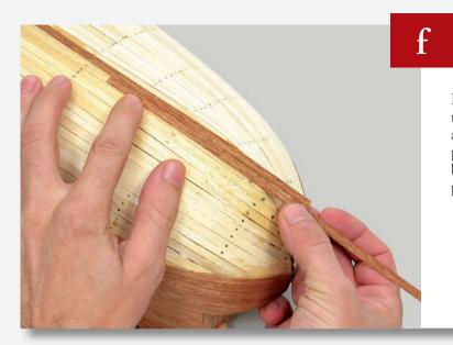
Place a second row of planks next to the row from the previous step, alternating the joins between the planks. Line them up with the base layer of planks to help you position them properly.
