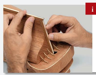
Position the stern post in place, up against the keel and slightly inside the hole at the base of the large
