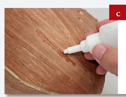
Pour superglue over the area to fix the dust. Repeat the filling process for all the cracks that remain.
