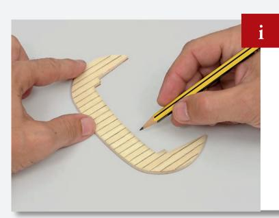
Turn the small stern deck piece over and cover the other side with any spare thin planks.
