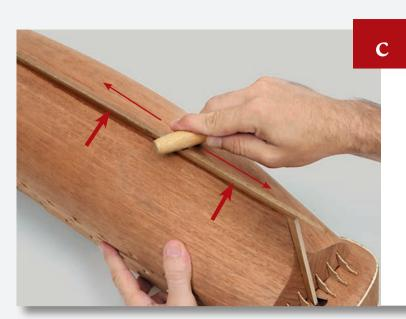
Continue to plank along the keel, using the planks from Page 217. Press along it to smooth the planks flat, and when the glue is dry, cut off the excess at the end.
