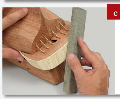
Then smooth the outer surface of the planks to create an even surface.
