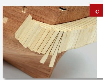
Because the stern assembly curves round, it may be easier to position the planks at an angle to match. Fill the gaps with shaped bits of plank, as you did with the hull.
