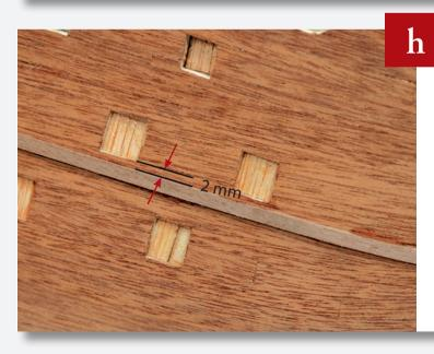
When gluing the wooden strip along the sides of the hull, make sure it rests 2mm below the gun ports.
