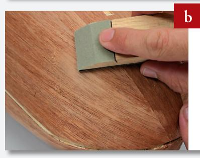
If you find a gap, gently sand the hull around it and fill it with the dust that you create.
