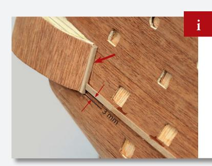
Cut a length of wooden strip to fit at the front of the stern assembly, and glue into place. Continue to glue wooden strips to the side of the hull in line with the strip you fitted in Step h. When you reach the stern, shape the end to an angle and glue it 3mm above the bottom of the wooden strip at the front, as shown.
