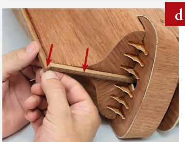
Cover the stern end of the keel, along with the stern post, with the same planks.
