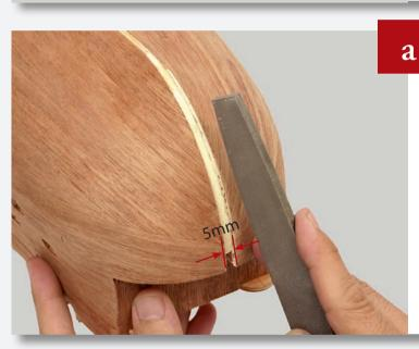
File the gap between the two sides of the hull along the false keel, so that the gap is 5mm wide.
