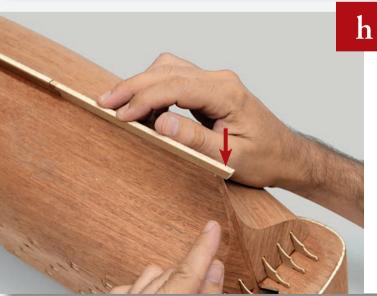
Place the last piece of the keel in the gap along the false keel. It will protrude past the stern.
