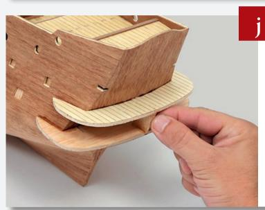
Test-fit the mid-sized stern deck piece in place and then place the spacer from Page 193 between the two stern deck pieces. Glue both into place.
