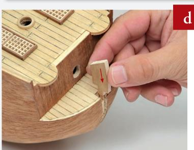
Test-fit the bowsprit support in place, as shown. Make any adjustments to the fit and smooth the surface. Then glue in place.
