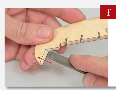
Sand the edges of the largest stern deck piece to smooth them. Shape the inner areas, as shown, so that they fit the hull better.
