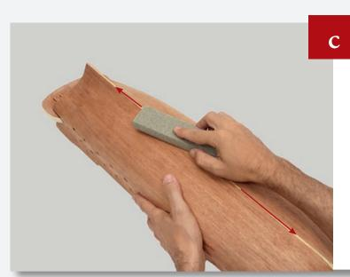
Sand along the bottom of the hull to level both sides of the false keel.
