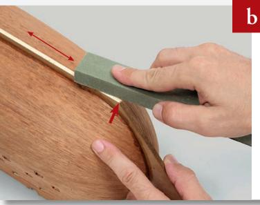
Sand the end of the plank where it comes into contact with the keel, so that the two are in line.
