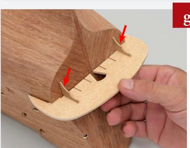
Remove two of the supports from the sheet and test-fit in the bottom of the stern deck piece and up against the stern, checking that the angle is correct.
