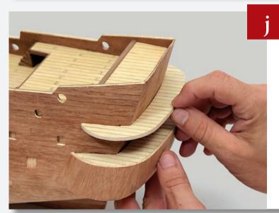
Glue the small deck piece in place, parallel with the lower decks.
