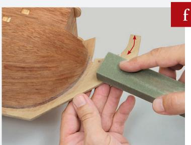
When the glue has dried, sand the stem, keel and stern post to remove any plank that runs over the width.
