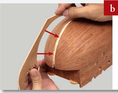
Test-fit the stem in the groove at the bow.
