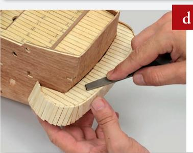
Once dry, cut away the parts of the planks that run past the edges of the deck pieces and smooth them so they are flush.
