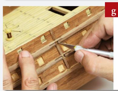
Cut away the space between each pair of marks made in the last step on each of the strips.
