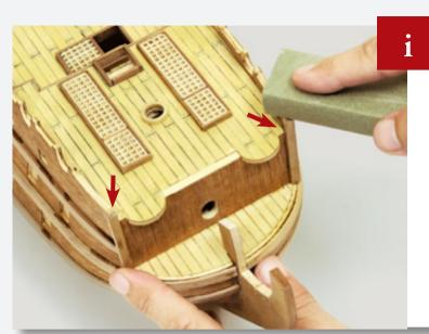
Repeat these steps for the other side of the hull. Smooth the upright lengths at the bow so they are in line with the tops of the bulwarks.
