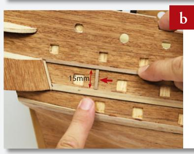
Cut a piece of 2 x 3mm wooden strip to about 15mm in length. Glue the wooden strip from the last step to the side of the hull, using the 15mm length as a spacer to keep the height accurate.
