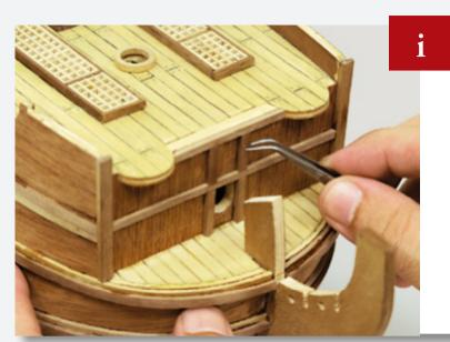
Using the remaining lengths of the 2 x 3mm wooden strips, cut four lengths, two to fit either side of the bowsprit hole and a further two to fit in line and above them.
