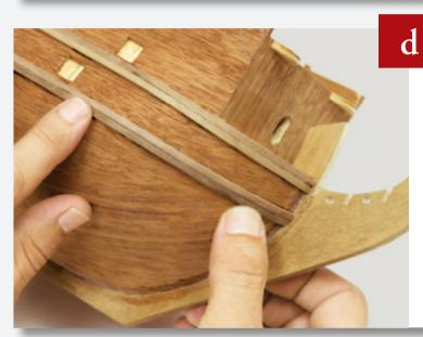
Begin placing a second set of wooden strips below the first.
