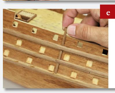
Cut three pieces of 2 x 3mm wooden strip to fit vertically between the horizontal strips, aft of the fifth gun ports from the bow.
