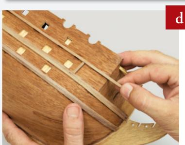
Continuing along the side of the hull, glue another wooden strip into place, again using the 15mm length to maintain the height.
