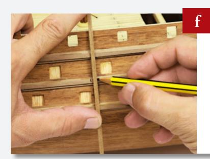
Hold a wooden strip over the three lengths from the last step and make a mark on each side of it on the horizontal strips, as shown.
