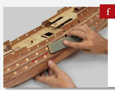
Smooth the surface of the wooden strips on both sides of the hull.
