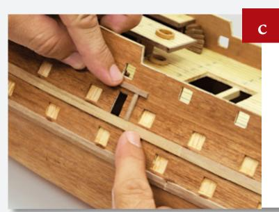
As you get to the end of the wooden strip, move the spacer to the end to maintain an even height.
