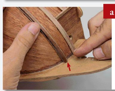
Cut a 2 x 3mm wooden strip to a length of 250mm and place it in the middle of the two strips, as shown.
