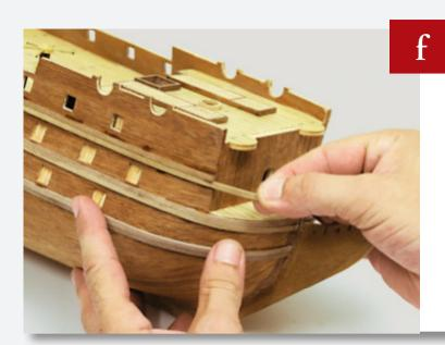
Continue along the side of the hull, gluing another wooden strip in place, flush with the one above.
