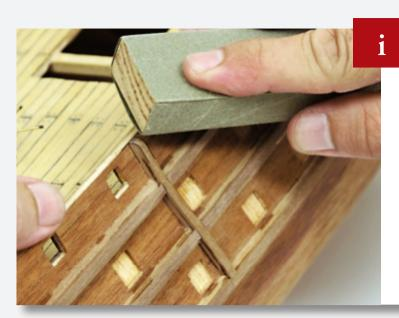
When the glue is dry, smooth the surface so that the wooden strips are flush at this point. Also, round the top of the strip.
