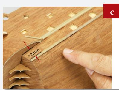
Continue placing wooden strips along the side of the hull. When you reach the stern, make sure that there is a gap of 12mm below the stern castle.
