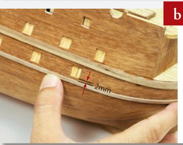
Continue to plank around the bow, keeping the wooden strip 2mm below the gun ports.
