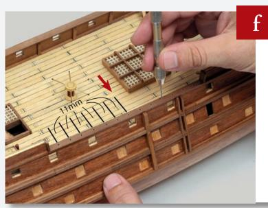
On one side of the ship, drill a series of shallow holes with the 0.75mm drill bit in the wooden strip along the bulwark of the main deck, 11mm apart.
