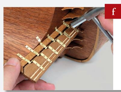
Position the rudder at the stern and nail into place, as shown.
