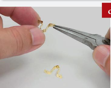
Shape three rudder fittings like those shown on the left; these will fit either side of the stern keel. The remaining three should be left straight, as they will have to be shaped to fit the hull.
