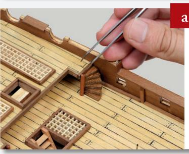
Hold the 3mm dowel on the main deck and cut a length equal to the height of the fore deck, then glue it into place alongside the stairs on the starboard side, as shown.
