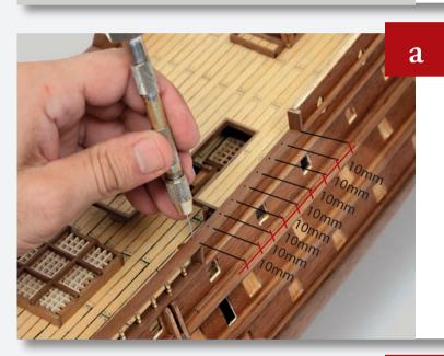
Locate the area shown, on the port side of the quarterdeck. Drill eight holes along the wooden strip, spaced 10mm apart.
