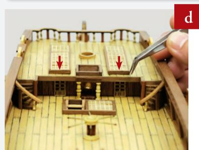
Glue two of the doors against the bulkhead, aligning them with the centres of the gratings above.
