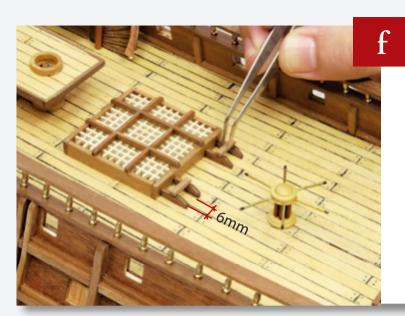
Cut four 12mm lengths of 2 x 4mm wooden strip and sand one corner of each to an angle. Glue in front of the hatch on the main deck with 6mm between them. Then cut two 12mm lengths of 2 x 2mm wooden strip and glue them onto the 2 x 4mm lengths, as shown.
