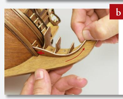
Glue the wider end of one of the frames above the middle wooden strip at the bow and along the bottoms of the beakhead bulkheads.
