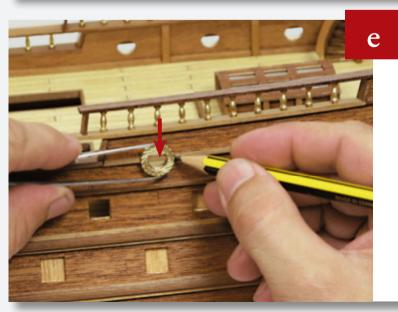
Hold one of the gun port rings over the first circular gun port from the bow. Mark either side of the ring on the wooden strip behind it. Then cut away the wooden strip between the two lines.
