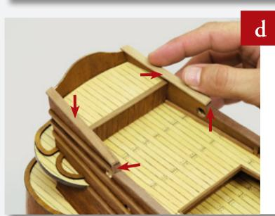
Cut two small pieces of 2 x 7mm wooden strip to fit vertically, then cut two longer pieces to fit horizontally, finishing at the stern.
