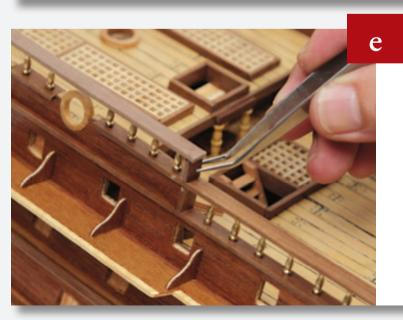
Cut and glue two lengths of 2 x 7mm wooden strip to fit below the strips glued in the previous step, as shown.
