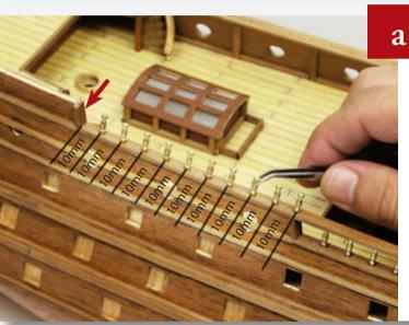
Cut a piece of 2 x 7mm wooden strip to fit at the point arrowed, and glue into place. Then measure ten points from the wooden strip, 10mm apart. Drill a shallow hole
