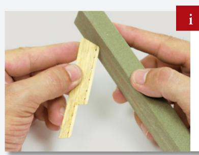
Continue to sand the chainwales, rounding the corners of the wooden strips slightly.
