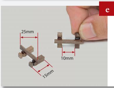
Cut four 15mm lengths of 4 x 4mm wooden strip and two 25mm lengths of 2 x 4mm strip. Shape the 15mm lengths the same way as the 35mm strips in Step a, and then position them 10mm apart. Glue the 25mm strip just below the grooved part, as shown.
