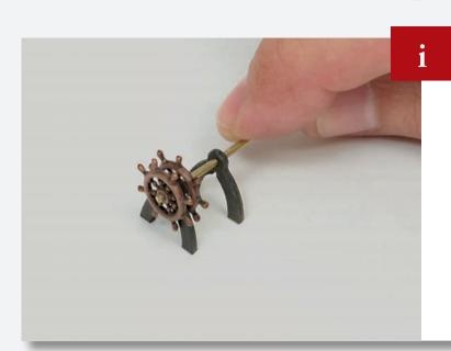
Hold a length of 1.5mm brass wire and place the two helm supports followed by the two helms onto it. When all the pieces are on the wire, push them to the end and apply glue. Once the glue is dry, cut away any excess wire.
