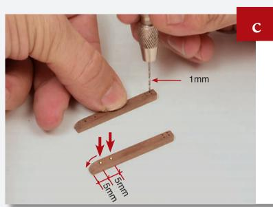
To make the davits, first cut two 50mm lengths of 4 x 4mm wooden strip. Drill four 1mm holes at one end of each, as shown in the photo, and then another two 1mm holes, one 5mm in from the other end and the other 5mm from that, and place a nail in each of these two holes. Then shape the end with the two nails in it so that it curves, as shown.
