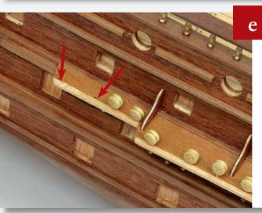
Leave the two holes at the stern end of the wale free because small deadeyes will be fitted into them at a later stage.
