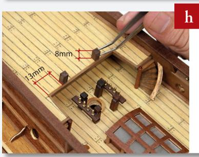
Cut two 8mm lengths of the 4 x 4mm wooden strip and glue into place on the quarter deck, 13mm in from the inner edges, as shown.
