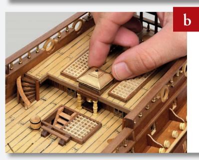
Test-fit the dome into place. Make any adjustments to the fit as necessary, and then glue the dome into place.
