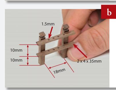
Cut two 35mm lengths of 2 x 4mm wooden strip. Position the two uprights 18mm apart and glue one 35mm length to them, 10mm from the base. Then drill four 1.5mm holes in the space between the uprights. Glue the other 35mm length 10mm above the first and drill another four holes, as shown.
