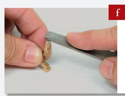
If the support doesn't fit, use a file to reduce the size. Keep test-fitting until the fit is correct.
