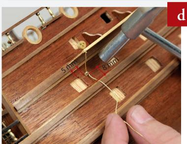
Feed the wire through the end hole of the fore chainwale. Insert a nail into the side of the hull below the chainwale, 5mm from the side of the gun port and 8mm above the wooden strip. Wrap the wire around the nail once then push the nail into the hull.
