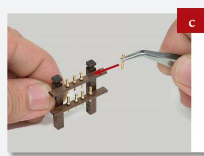
Stain the pinrail assembly and then glue eight pins into the holes, as shown.
