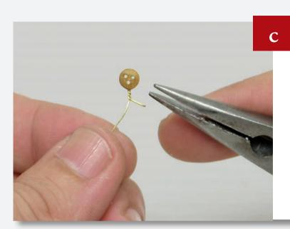
Cut a 100mm length of brass wire, then, as shown, wrap it around one of the deadeyes. Make sure the holes of the deadeye are positioned as in the photo.
