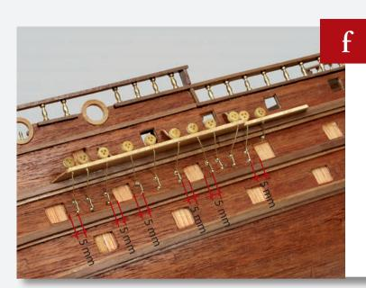
Repeat Steps c-e to fit a further ten deadeyes to the fore chainwale. Make sure that there is always a minimum of 5mm between any nails and gun ports, as shown.
