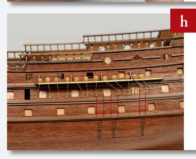
Following the same process used with the fore chainwales, fit twelve deadeyes to the main chainwale, as shown, leaving a minimum of 5mm between the nails and gun ports, or 10mm where specified.
