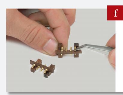
Stain the two pinrail assemblies. Drill four holes in each of the 2 x 4mm strips, as shown, then glue a pin into each of the holes.
