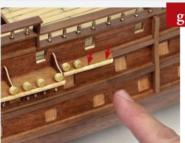
The two remaining holes at the stern end of the fore chainwale should be left, because small deadeyes will be fitted to them at a later stage.
