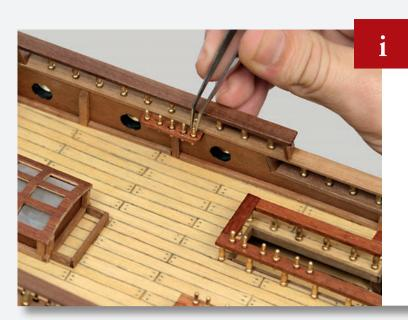
Stain the pinrails and then glue pins into the holes.
