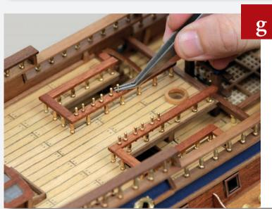
Glue a pin into each of the holes drilled in the previous step.
