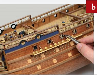
Then glue gun port frames to the main deck gun ports on the port side.
