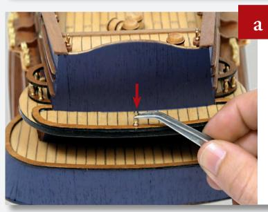
Mark the centre point on the edging of the upper deck at the stern, drill a shallow hole and glue a column in place.
