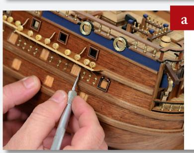
Test-fit the gun port frames in each of the ports, adjusting the ports if necessary.
