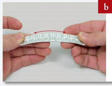
Bend the lower window casting slightly to match the curve of the transom, with the smooth side underneath on the inside of the curve.
