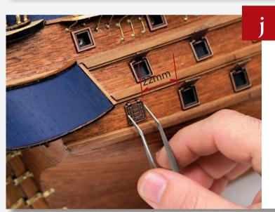
Scrape another small area, aft of the last gun port on the lowest deck. Then glue a complete gun port in place, with a gap of 22mm between it and the next gun port, as shown. Repeat for the other side of the hull.
