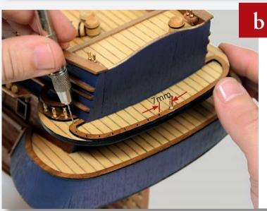
Drill a series of nine holes on the port side at 7mm intervals from the central column.
