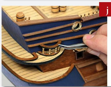
Test-fit, prepare and glue the edging pieces into place, resting on top of the columns from Step h, on both sides of the hull.
