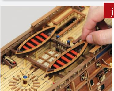
Apply some glue to the gaps between the 5mm lengths and fix the lifeboats in position, as shown.
