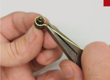
Take the 60mm length and form a loop at one end, around one of the lanterns.
