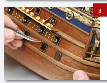
Assemble and place a gun port lid over the remaining gun port on the starboard bow.
