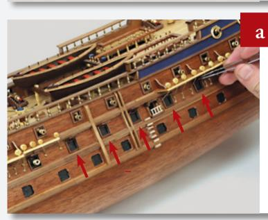
Assemble five gun port frames and lids and glue them in place over the gun ports of the gun deck on the port side, as indicated by the arrows.
