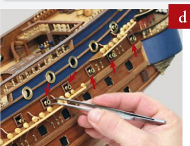
Drill five holes (arrowed) along the main deck and glue a dummy gun into each of them.
