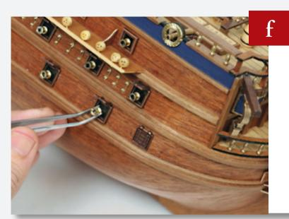
Drill a hole and fit a dummy gun into the gun port at the bow on the lowest deck on the starboard side.
