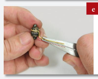
Angle the wire down and then bend it out so that it faces away from the lantern, as shown.
