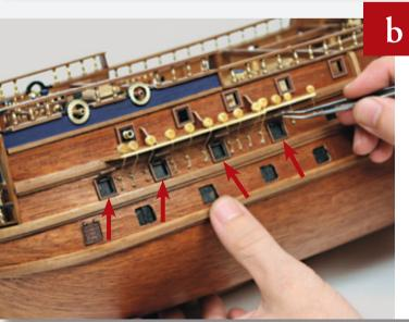
Then place four assembled gun ports over the first four ports of the port gun deck (arrowed).
