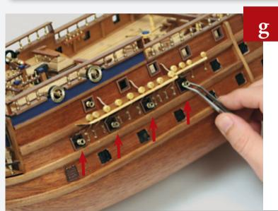
Drill four holes in the first four gun ports of the gun deck on the port side and glue a dummy gun into each one.
