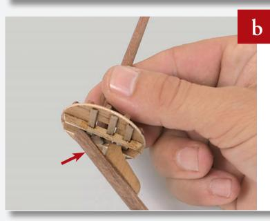
Place the spritsail topmast into the hole of the maintop, resting on the bowsprit, and glue it into place.
