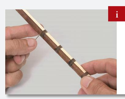
Use the brown thread (18) to create the six bindings (22), as indicated on the plan. Each binding is six turns of thread wide.
