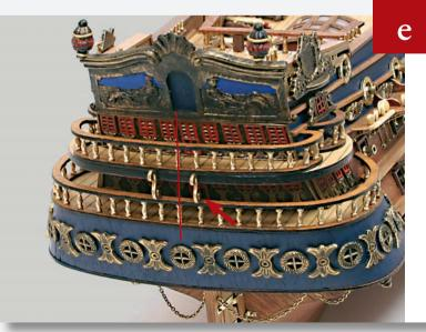
Glue another ornament (arrowed) to the starboard side of the central columns (red line).
