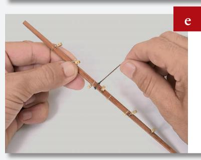
Take a piece of 0.5mm brown thread (part 18), and tie one end in the centre of the yard (17). Leave the free end loose to attach to the bowsprit at a later stage.
