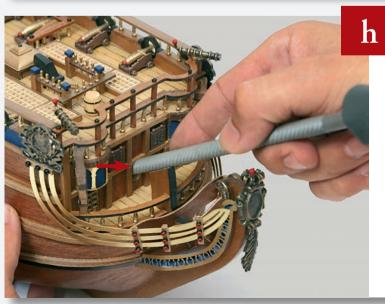
Clear the hole at the bow where the bowsprit fits, as the ends of some wooden strips or planks may be obstructing the hole.
