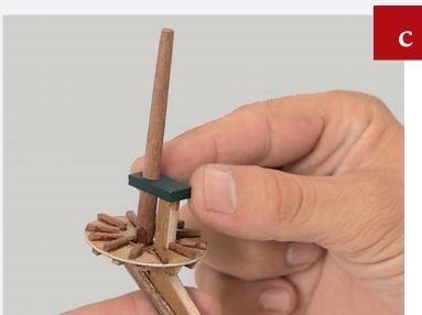
Place the lower mast cap over the topmast and slide it down until it comes into contact with the top of the knee, then glue it into place.
