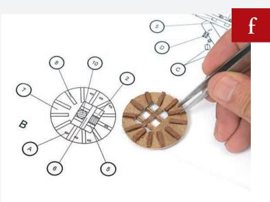
Turn the maintop over and glue the ribs (part 8) into place.
