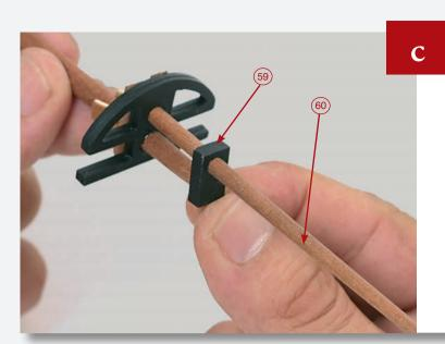
Glue the main topgallant mast with the upper mast cap into the crosstrees of the main topmast, and glue into place.
