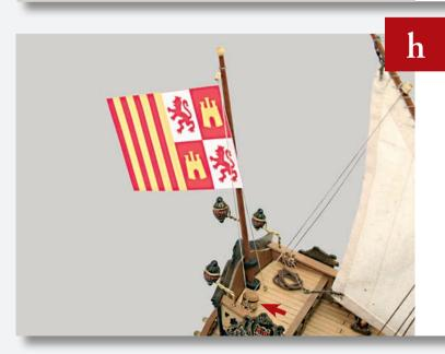
Hold the flag in the position shown and pass the upper length of thread through the hole in the block at the top of the flagpole. Pull the thread down and tie it off to one of the pins (arrowed). Tie the other end of the thread to the eyebolt in front of the flagpole.
