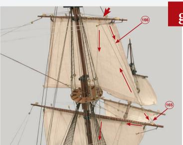
Using the photo and figure G on the rigging plan as guides, attach the sheets (165) and the clewlines (166) to the fore top yard and
