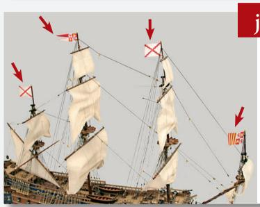
Prepare the other flags in the same way as in Steps f and g. Those with a cross should be attached to the foremast and the mizzenmast, the rectangular flag to the mainmast and the remaining flag to the bowsprit.
