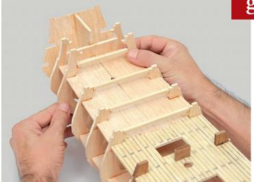
After cutting the beam, glue it in place. Repeat this operation for beams 10, 11 and 12.
