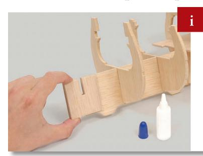
Following the same process as in Steps g and h, glue the other false keel reinforcement into place.
