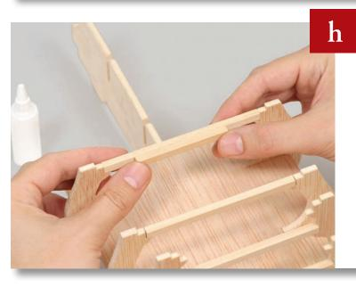
Cut a 70-mm-long strip of wood and glue it in the center of the beam of Frame 6. Make sure it is perfectly aligned and does not protrude either above or below the existing beam.
