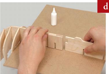
Once dry, apply glue to the new piece of false keel, then insert it between the two reinforcements until it is in contact with the previous false keel. Do this on a flat surface, so that they remain aligned along the top edge.
