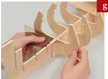
Make sure that the frame dries at a right angle to the false keel.
