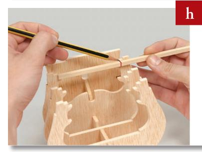
Take the 5 x 5-mm strip and position it across the gap in Frame 2, as shown. Mark the length of the gap on the beam and cut the beam at the mark. Repeat this process to make a lower beam that will fit as shown on the next page.
