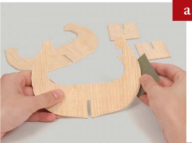
Smooth the frames and reinforcements with sandpaper to remove any burrs.
