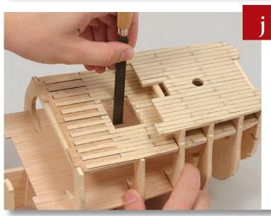
Smooth the ends of the section beam you just removed.
