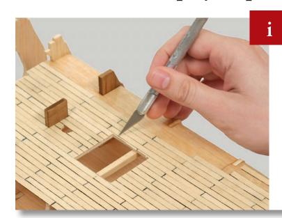
Stop planking when your deck reaches the stage shown in the photo. Cut away any planks that cover the holes in the deck.
