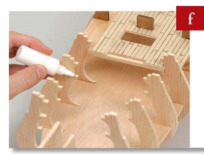
Apply glue to the lower ledges of Frame 10, as shown in the photo.
