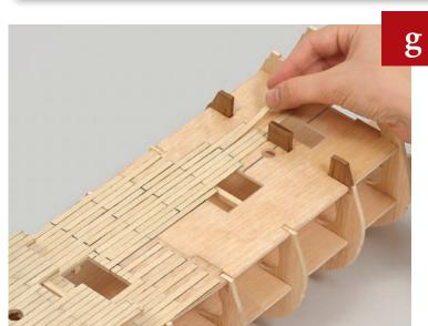
Cut the planks to a length of 70 mm and mark the edges as with the previous planks. Start to fix the planks to the deck by placing the first one along the line drawn in Step d, and the next in the gap between the planks of the previous part of the deck.
