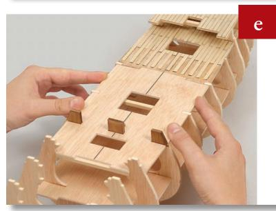
Position the deck on the frames to test-fit, and adjust if necessary.
