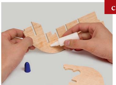
After ensuring that the pieces fit, remove Frame 2 and apply glue to both sides of the keel, below the second slot.
