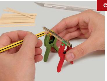
Cut the planks to a length of 70 mm. You will get two lengths from each strip, with some likely left over. Then take 10 pieces, hold them with their edges aligned using clamps, and blacken the edges using a pencil or a black marker.
