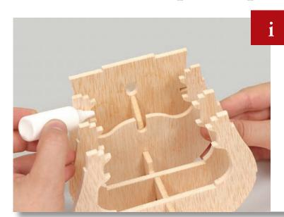
Now apply glue on the joints where the beams will be placed on Frame 2, as shown in the photo on the left.
