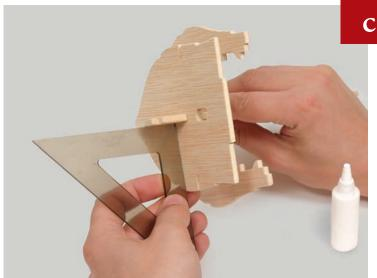
Using a triangle or similar straight edge, make sure the two pieces are at right angles. Hold them in place until the glue is dry.
