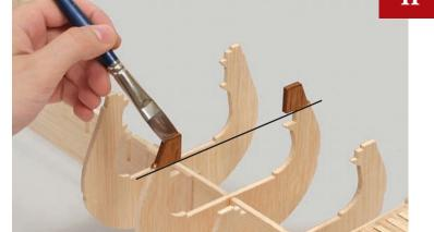
The top of Frame 8 protrudes through the main deck, so it is best to stain it at this point. Use a brush to stain the area above the black line as shown, working with the grain of the wood.
