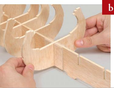
Test-fit Frame 6 in its corresponding slot, then glue into place, ensuring that it dries at a right angle to the false keel.
