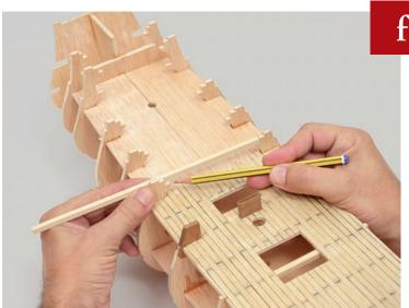
Take one of the 5 x 5-mm strips previously supplied and mark the length needed to fit across the ledges on Frame 9.
