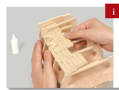
Test-fit the port bow deck in place. Then apply glue to the lower beams of Frames 2-6 and glue the deck in place.
