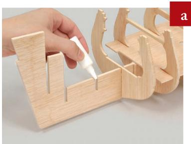
Smooth the deck and frame with sandpaper to remove any splinters. Then apply glue to the 11th slot of the false keel.
