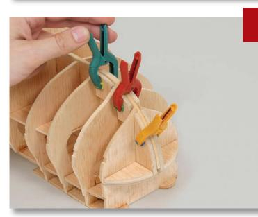
Use clamps to hold the false keel reinforcements in place while the glue dries.
