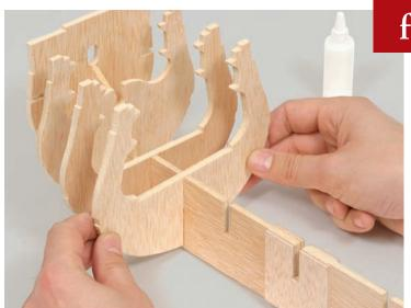
Now test-fit and glue Frame 4 in its position on the false keel, as shown.
