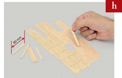
Cut planks 60 mm long and use them to plank the stern deck, overlapping the joints in the same way as before.
