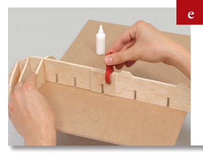
Hold the reinforcements firmly against the new false keel until the glue is completely dry.
