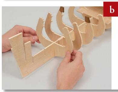
Place Frame 10 in place in the false keel, holding it as it dries, and ensuring that it is at a right angle to the keel.
