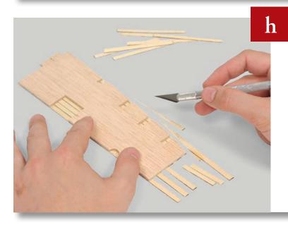
Once dry, turn over the deck and cut away any planks that extend past the edge and the three large notches in the side, as demonstrated in the photo.
