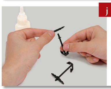
Apply a drop of superglue to the top end of the anchors, then insert them into the hole of the stock so that they sit at right angles. Support them so that the parts aren't pushed out of alignment while you wait for the glue to dry.
