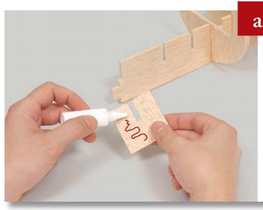
Smooth all the pieces of wood with sandpaper to remove any splinters. Proceed gently to avoid damaging them. Then apply glue to the false keel reinforcement, in the area shown in the picture.
