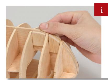
Now glue the remaining reinforcements flush with the false keel, on both sides, between the first and second frames and the second and third frames.
