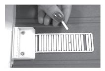
1. Remove two pins from the frame.
