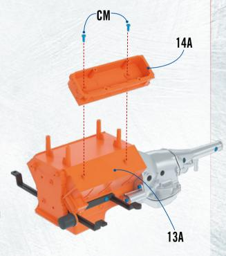
ATTACH the left bank cylinder head 14A (indicated with the letter "L" on the bottom) to the left side of the assembled engine block. Ensure that it is facing the same way as that shown in the illustration, then fix in place with two type CM screws.
