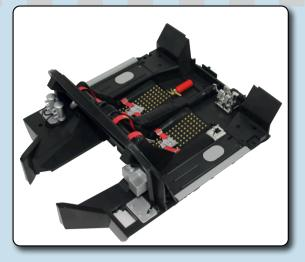
STEP 30-2 Install the steering support in front of the pedals. Secure it with two FP01 screws.
