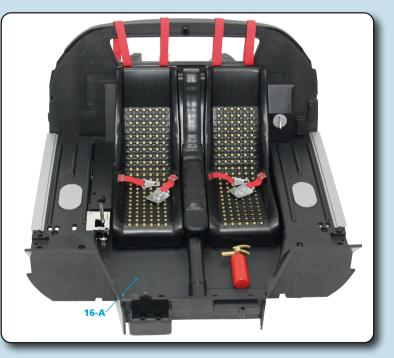
**STEP 27-9** Fit the seats into the centre of the floor, as shown, inserting the posts into the corresponding holes.
