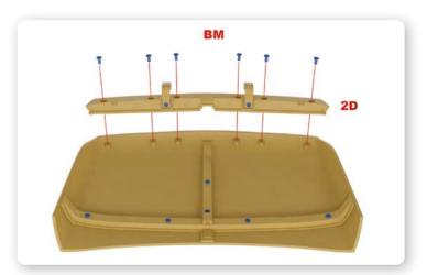
Take the assembly from Step 1 and place it onto the six posts towards the front of the bonnet. Fix in place with six BM screws.
