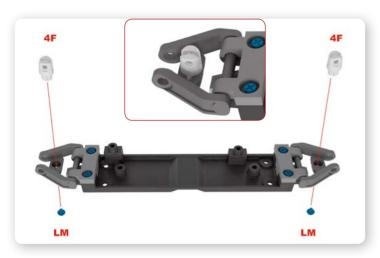
3 Insert the lower shock absorber mounts (4F) into the holes in the wishbones. Secure them in place with LM screws.
