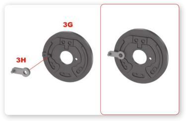
4 Mount the handbrake actuating lever (3H) onto the indicated pin of the brake plate (3G).
