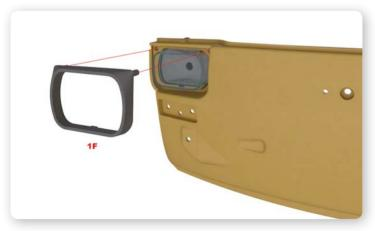
5 Fit the right headlight frame (1F) over the lens from the outside of the front panel.
