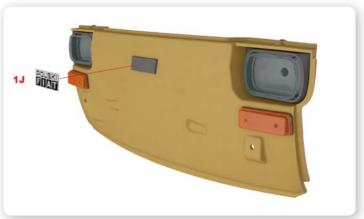
**8** Remove the backing from the front badge (1J) and fix it onto the front badge base.
