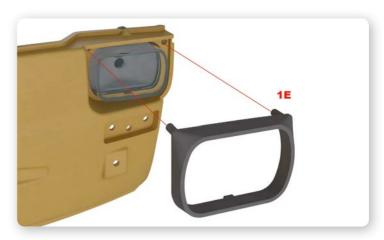
**2** Push the left headlight frame (1E) over the lens from the outside of the panel.
