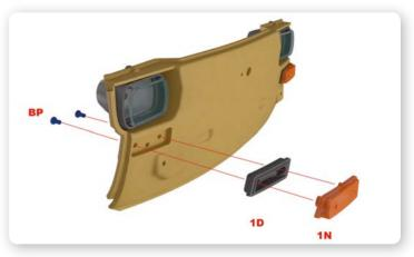
6 Secure the right front indicator housing (1D) and the right front indicator lens (1N) to the front panel with two BP screws.
