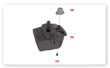
**3** Fix the carburettor to the engine block upper (5A) with a CP screw. It will only fit in one orientation.
