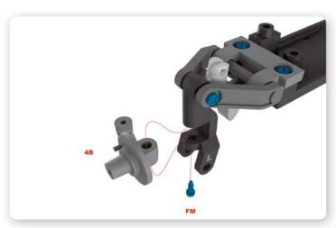
5 Fit the left wheel hub (4B) into the opening of the left kingpin. Secure in place with an FM screw.
