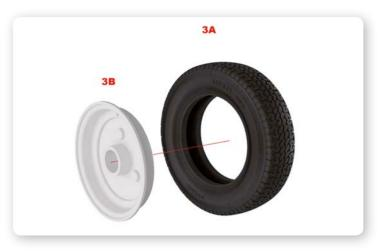
1 Start the wheel assembly by inserting the outer wheel rim (3B) into the tyre (3A).
