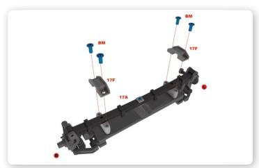
4 Fix the spring clamps over the leaf spring, to the mounts, with BM screws.
