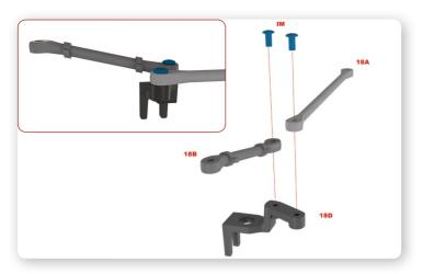
Connect the tie rod (18A) and the left tie rod (18B) to the idler arm (18D) with two IM screws. Make sure that the left tie rod is angled upwards.
