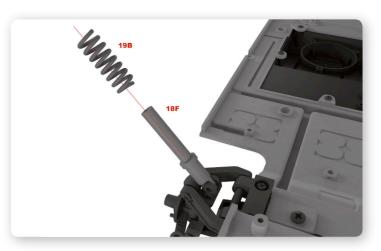
2 Slide one of the shock absorber springs (19B) onto the right shock absorber.
