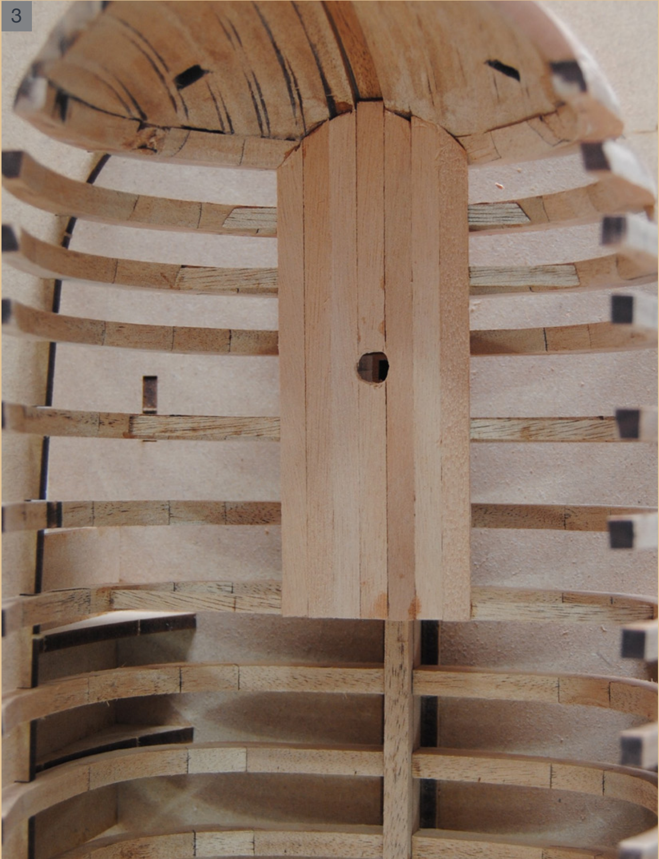
3 The bow planking correctly positioned.
