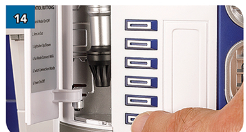
Read the next two pages so you are familiar with how to control R2-D2, then press the bottom button (Power On/off) on his front panel. He will jerk forward about 2cm to calibrate his motors, rotate his head in both directions, make a noise and illuminate status displays to indicate that he is ready for action.
