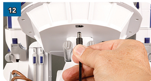
Plug the mains adaptor into R2-D2. Plug the other end into the mains and turn it on. Leave it for a couple of seconds, then turn off and unplug both ends. This is a protection procedure to activate the battery, and without doing this, R2-D2 won't turn on. You do not need to repeat this process, and in future the adaptor is only used to recharge the batteries. If R2-D2 is turned on, his front red/blue status light will change colour and flashing sequence to indicate the charge level (see the online User Guide for details).
