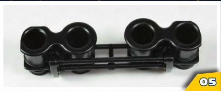
STEP 05 Fit the left intake ducts to the other side cover, in the same way as the right.
