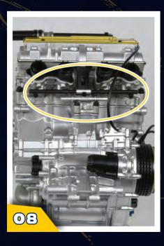
STEP 08 This is how the return rod should look when in position.
