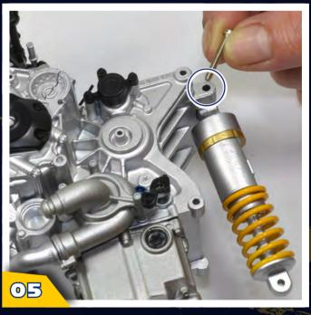
**STEP 05** Insert a type P screw through the aligned holes.
