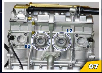
STEP 06 Take the two gaskets marked R2 and L2. These match the points on the engine that are marked the same.
