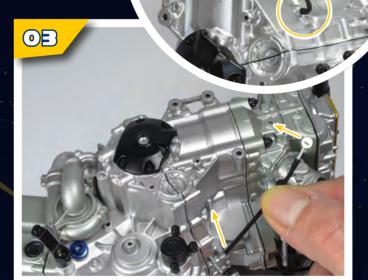
STEP 03 Now fit coupling B and the tube to the indicated points on the left-hand side of the engine.
