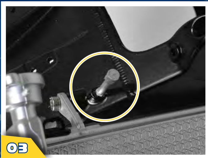
STEP 03 Then place the second limit switch into the circled hole in the right side of the frame.
