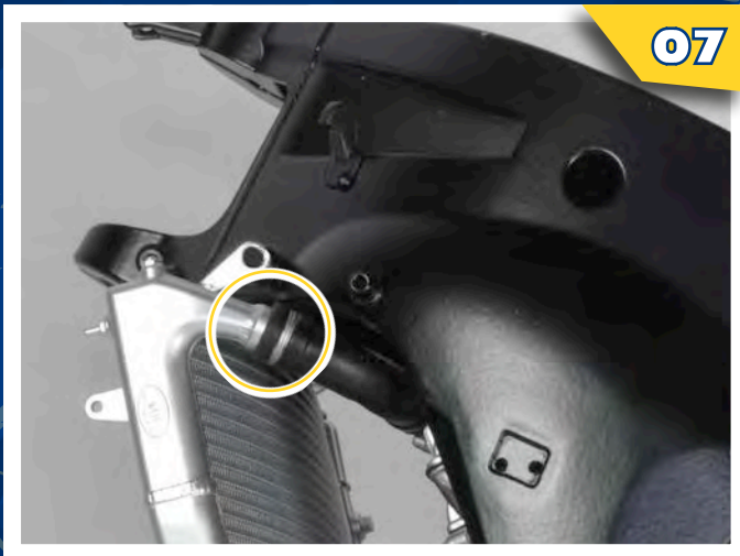
STEP 07 Connect the top of the radiator to the hose, as shown.
