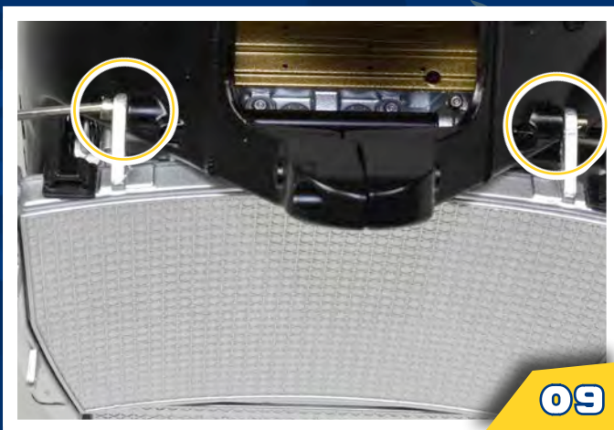
STEP 09 Secure the top of the brackets to the frame with two type V screws.
