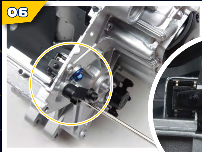
STEP 06 Gently tighten the screw into place, ensuring that the parts stay in position. The inset shows how the assembly should look.
