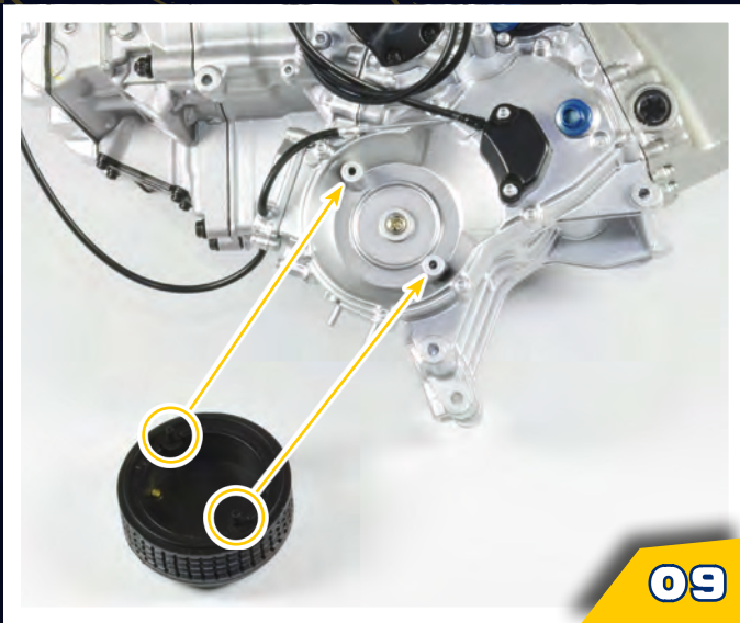
STEP 09 Retrieve the engine block and insert the two pins on the reverse of the clutch (circled) into the two holes in the side of the engine block (arrowed).
