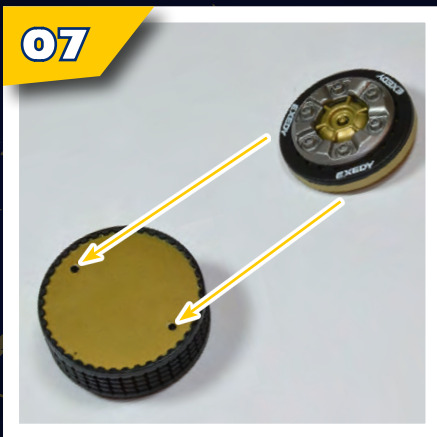
STEP 07 Retrieve the clutch assembly from Stage 33. The two pins on the reverse of the clutch cover fit into the two indicated holes in the clutch.
