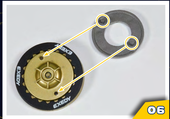
STEP 06 Fit the clutch flange onto the clutch cover, inserting the pins into the holes.
