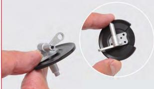
**STEP 6-B** The backplate and steering knuckle should look like this after assembly.
