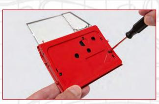
**STEP 10-I** Fix the inner panel to the door with three SD04 screws.
