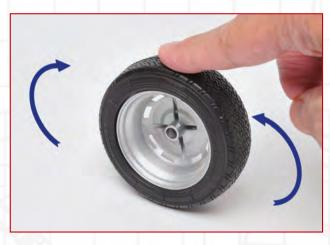
**STEP 7-D** If necessary, rotate the wheel, pressing on the tyre so that it is perfectly positioned on the rim.
