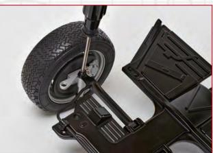
**STEP 14-K** Turn the assembly over and secure the track control arm with an SD08 screw.
