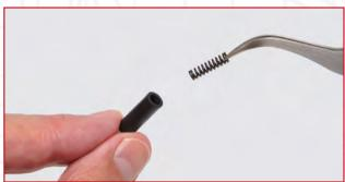
**STEP 6-I** Fit the internal damper spring (6-8) into the shock absorber body (6-6).
