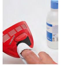
**STEP 8-A2.** Take the engine cover you assembled in Stage 3, together with the stickers supplied. Before using the stickers, clean the number plate with a cloth moistened with a little alcohol (such as methylated spirits) to ensure the best adhesion.
