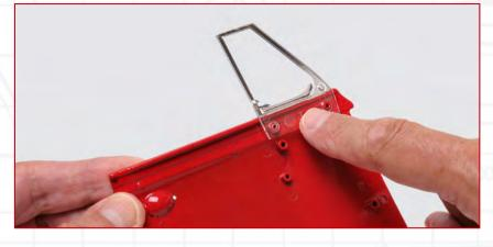
**STEP 8-C** Fix the quarterlight to the door panel with two SD05 screws.
