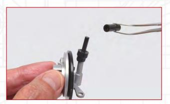
**STEP 6-J** Fit the assembly from Step 6-I over the shaft of the shock absorber piston.
