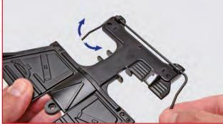
**STEP 13-F** After fixing both supports, check that the anti-roll bar is free to pivot up and down as shown.
