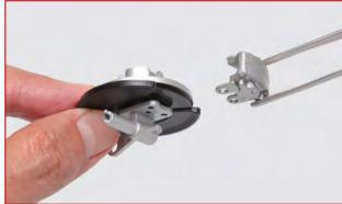
**STEP 6-D** Fit the caliper (6-2) over the brake disc and the recessed portion of the backplate.
