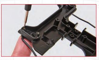
**STEP 13-D** Turn the assembly over and fix the support with an SP11 screw.
