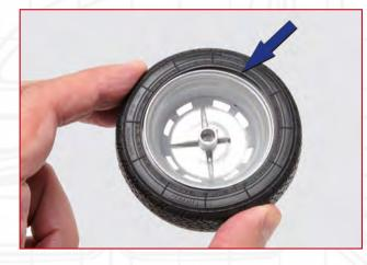
**STEP 7-C** Check that the tyre beads are perfectly seated on the rim all the way round.
