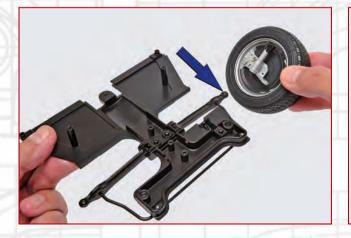
**STEP 14-J** Place the bottom of the left steering knuckle on the end of the left track control arm.
