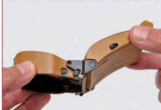
**STEP 11-H** Fit the recesses in the recliner mechanisms over the pins, as shown.
