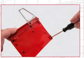
**STEP 9-B** Fix the hinge to the door with two SD07 screws.
