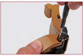
**STEP 11-J** Fix the arms of both recliner mechanisms to the seat base with two SP10 screws.
