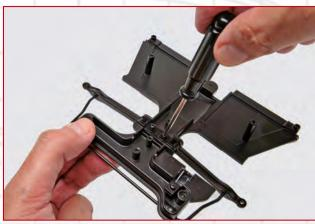
**STEP 14-H** Fix the pivot mounting to the subframe with two SD04 screws.
