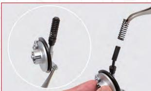
**STEP 6-K** Fit the front suspension spring (6-9) over the shock absorber.
