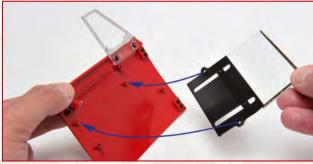
**STEP 9-1** With the window in the raised position, align the assembly with the inside of the door panel so that the two lugs on the regulator will fit over the mounting holes indicated.
