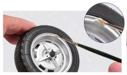
**STEP 12-A.** Take the front wheels you assembled in Stages 2 and 7. Using a very fine brush and mid grey paint, pick out the balance weight on the rim as shown. It is very important to use very little paint on the brush to avoid marking the rim next to the weight.
