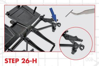
Slide the shock absorber rod (26-7) into the damper tube.
