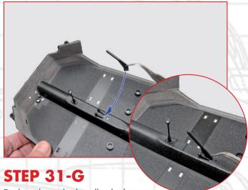
Fit the tab on the handbrake lever (31-2) into the long slot, making sure it goes all the way in.
