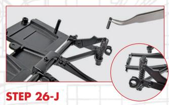
Fit the internal damper spring (26-6) inside the rear suspension spring and over the damper tube.
