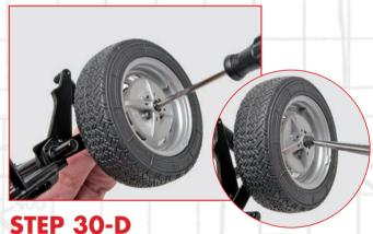
Fix the wheel to the stub axle with an SD02 screw, then press a VW into the hole to cover it.
