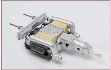
The main assembly of the engine/transmission is complete and should look like this from below.
