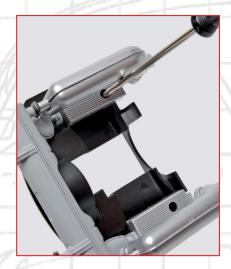
**STEP 35-L**Secure the cylinder head section with another SP13 screw.
