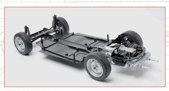
The main assembly showing the engine and transmission in place in the chassis.
