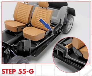
Check that the rear end of the passenger compartment is fitted flush on both sides.
