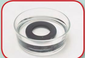
To make it easier to fit the tyre onto the wheel, either heat it slightly with a hair dryer or immerse it in hot water for a few minutes. Doing this will make the tyre softer and more pliable while you fit it, and it will harden again as it cools.
