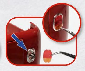
STEP **112-D** Place the lens (112-5) into the light from the outside.
