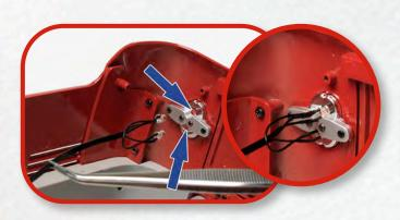
STEP **112-E** Insert the LEDs (112-8) into the indicated holes in the rear of the light.
