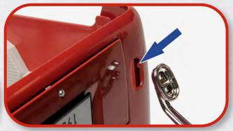
STEP **112-B** Fit the left rear light (112-4) into the corresponding space in the body.
