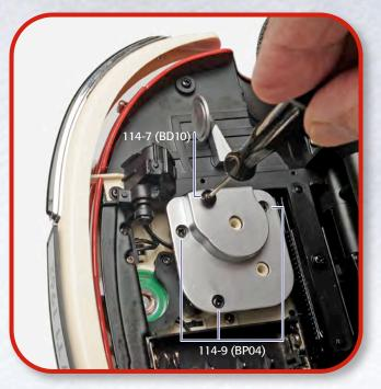
STEP **114-F** Secure the gear case to the chassis with three BP04 screws (114-9). Tighten a BD10 screw (114-7) into the end of the pinion.
