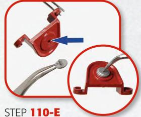
Insert the pin on the inside of the fuel tank cap (110-10) into the hole in the support (110-9).
