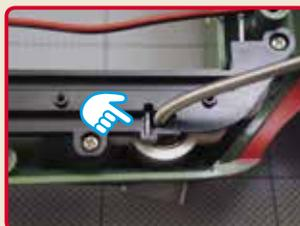
Check that the 4 guide pins are correctly installed to the slide rail.
