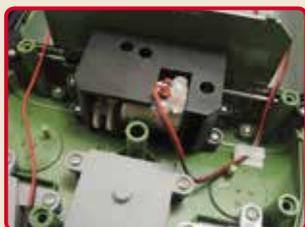
Check that the motor unit is tightened securely with the 3 screws.
