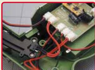
Because the raising of the unit is detected by the upper limit switch installed to the slide rail, check the installation status, wiring and connectors of the upper limit switch.
