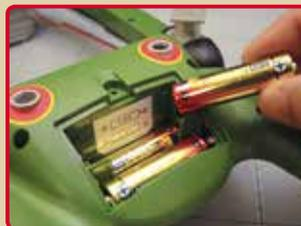
Check that the switch on the unit is OFF. Insert 3 new AA batteries facing in the correct direction. Remove the 15 screws that connect the top and bottom of the unit.
