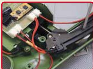
Because the lowering of the unit is detected by the lower limit switch installed into the slide rail, check the installation status, wiring and connectors of the lower limit switch.
