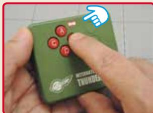
The remote control does not have an ON/OFF switch. By pressing buttons A to D, the light on the remote control will turn on in red meaning that the unit's functions can be operated.
