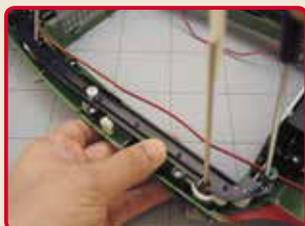
Check that the right and left slide rails are tightened securely with the 6 screws.
